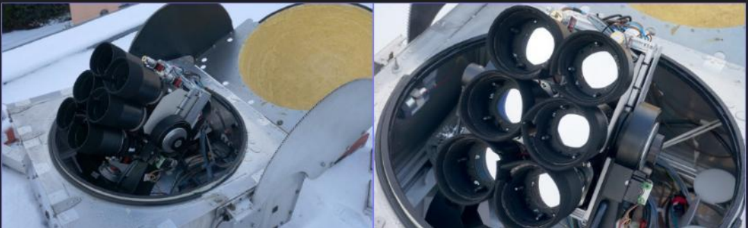
H \alpha instruments (3 and 4, the four smaller lenses) and the continuum cameras (5a to 5c, the three large lenses).
