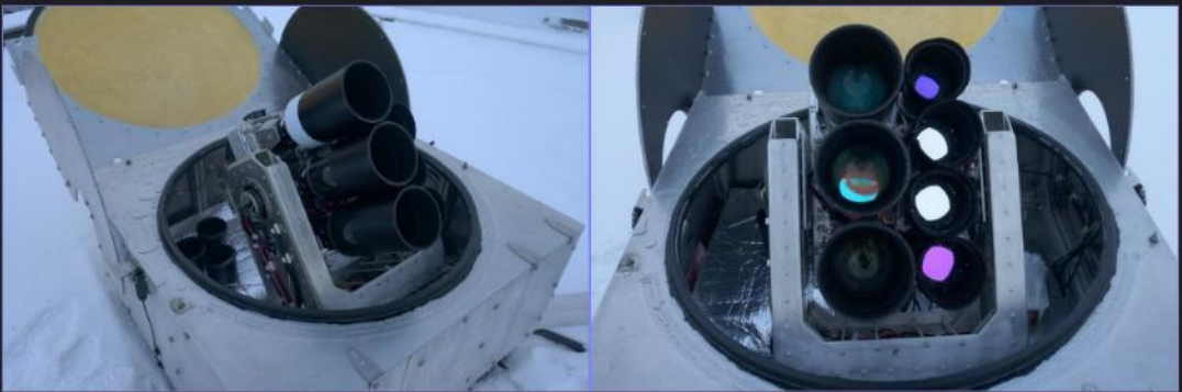
H \alpha instruments (3 and 4, the four smaller lenses) and the continuum cameras (5a to 5c, the three large lenses).
